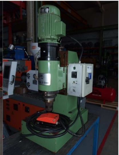
Remachadora orbital radial 0-10 mm. LAU-NIK 0-10 mm. Ref: 17830
